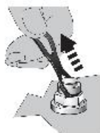
拆下运输保险（橡胶圈） Removing the transport fixture (rubber ring)
