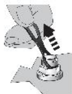
拆下运输保险（橡胶圈） Removing the transport fixture (rubber ring)
